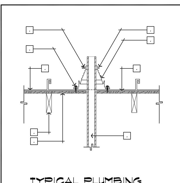
TYPICAL PLUMBING VENT STACK DETAIL A3.02 SCALE: 1/2" = 1'-0"
